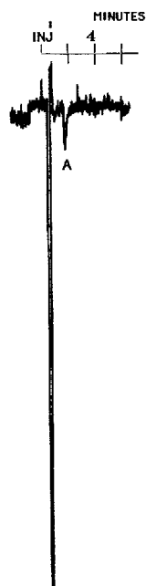
Fig. 5. Chromatogram of 0.2 ppm fluoride ion with IEC-IPD. Conditions as in Fig. 4.
